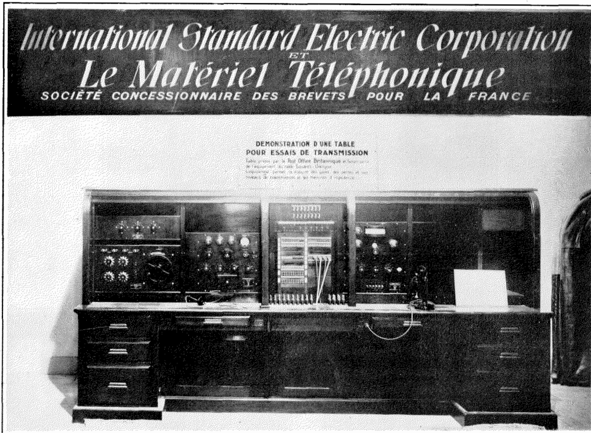
Figure 17—Repeater Station Test Desk
